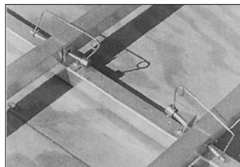
42" railing locked in "down" position.
