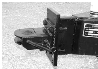
The safety pin must always be used on a coupler hitch when towing.
