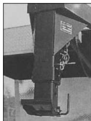
Adjustable ball coupler gooseneck hitch. Make sure latch is closed before towing.
