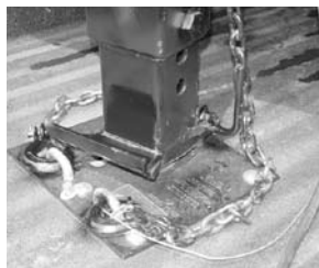
Gooseneck hitch shown with safety chains and breakaway cable affixed to the tow vehicle. Always tow with the safety pin locked as shown. (5th wheel must have safety chains attached to vehicle also!)
