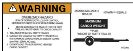
Warning Overload Hazard Label – Figure 1-2
